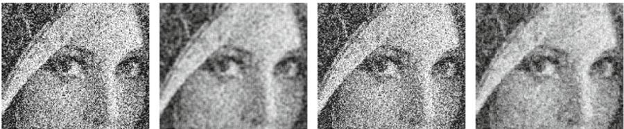
(m)  $\sigma = 0.24$  (PSNR: 13.2, SSIM: 0.09) (n) Lee-filter (PSNR: 19.8, SSIM: 0.24) (o) Bilateral filter (PSNR: 13.9, SSIM: 0.08) (p) Proposed (PSNR: 22.1, SSIM: 0.35)
